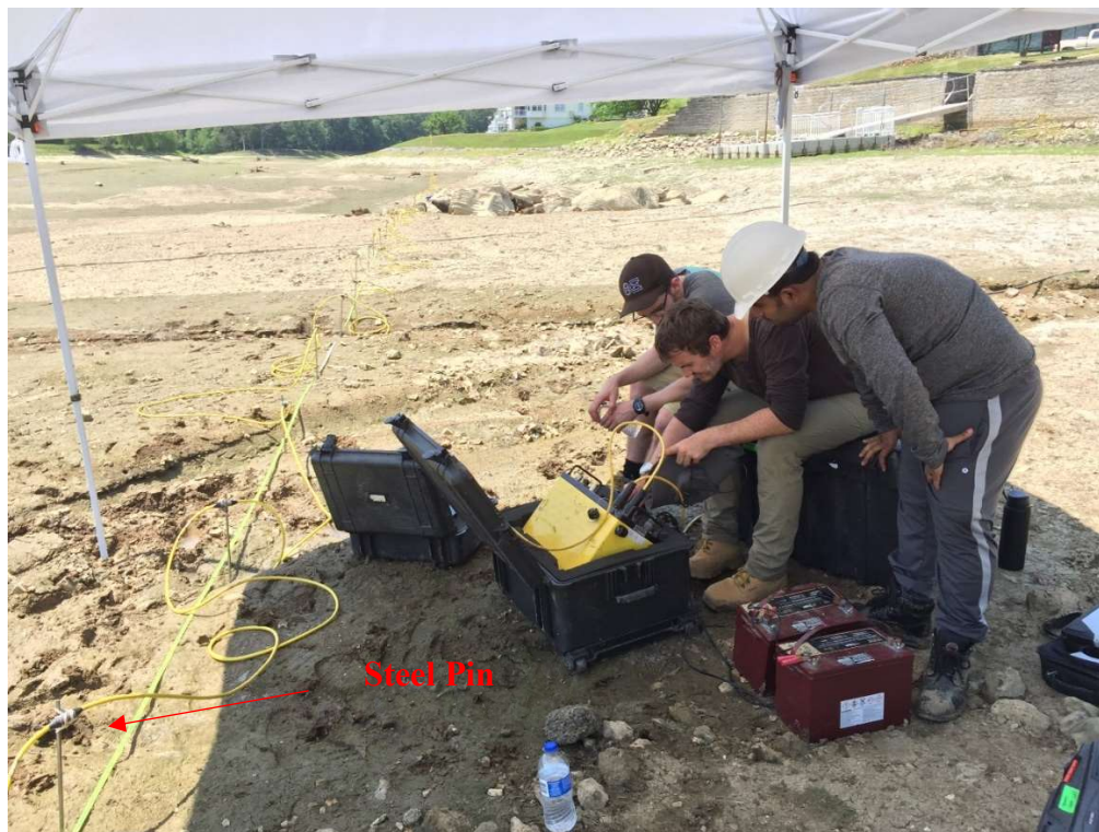
Figure 4.3. The setup of an ERT system.
