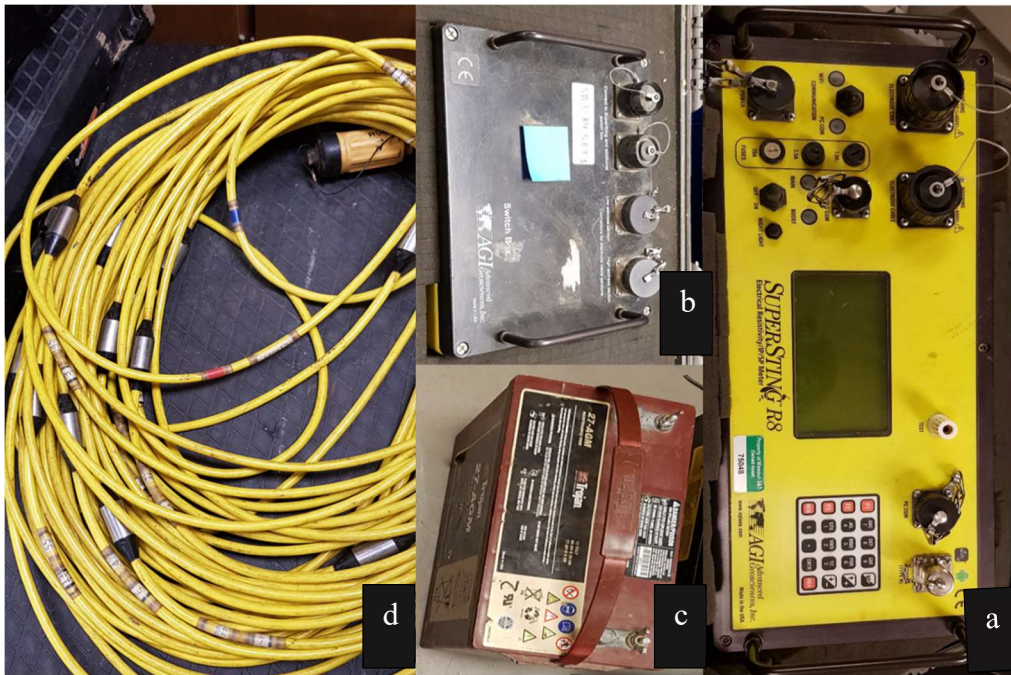
Figure 4.2. Equipments of ERT survey: a. supersting control unit; b. switch box; c. battery; d. survey cable.
